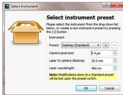
Figure 6: Initial set-up of Swordfish based on the microscope used
