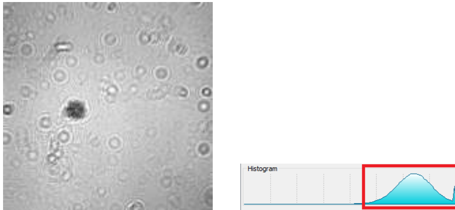
Figure 11: An over exposed hologram, and the histogram associated with over exposure.
