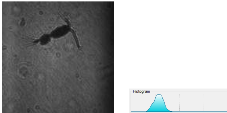
Figure 12: A properly exposed hologram, and the associated histogram.
