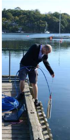
Figure 16: Deployment of the Submersible from a wharf
