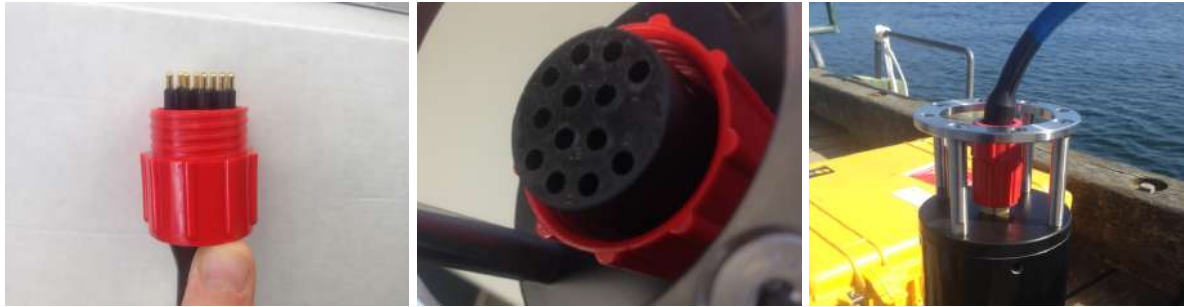
Figure 12: Locking sleeve on both the cable (left panel), the microscope (center panel) and connected (right panel)
