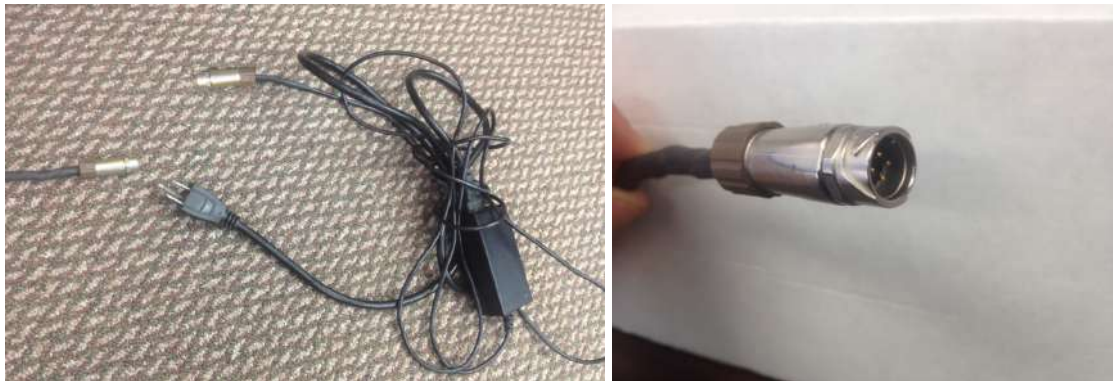
Figure 15: Connecting the power. In the left panel connecting the microscope power to the included 12VDC power cord. The right panel shows a close-up of the power connector from the microscope.
