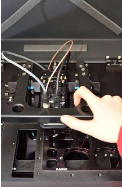
Figure 25: Moving the Camera pull bar forward.
