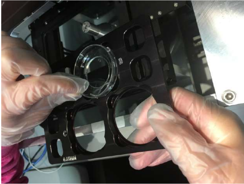
Figure 23: Placing the MaTek dish in the Sample inset.
