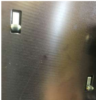
Figure 16: The two Interlocks. The left Interlock is to trigger that the Lid is closed, and the right Interlock is to trigger that the Camera pull bar is in the forward position.
