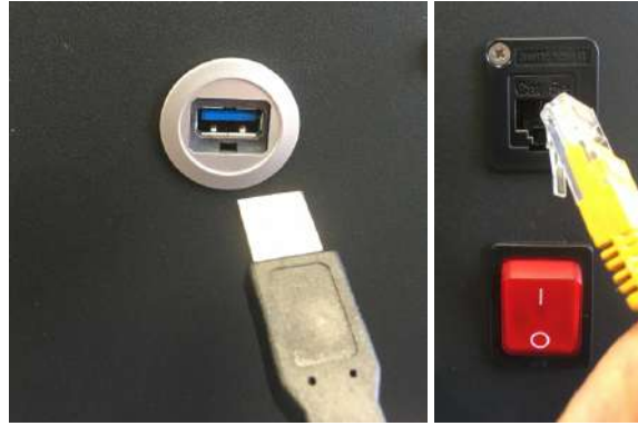
Figure 18: Connecting the USB (left) and the Ethernet (right) to the HoloScan.
