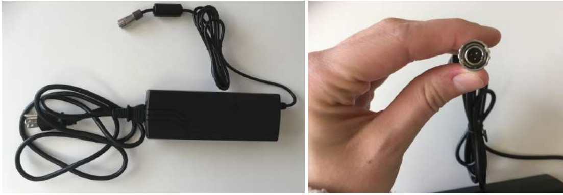
Figure 8: Power supply for sample stage (3 prong).
