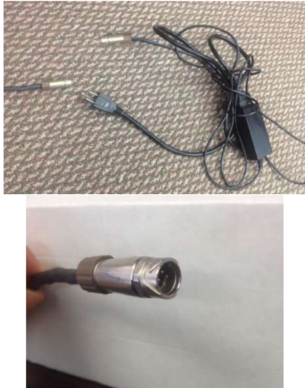
Figure 12: Connecting the power. In the left panel connecting the microscope power to the included 12VDC power cord. The right panel shows a close-up of the power connector from the microscope.
