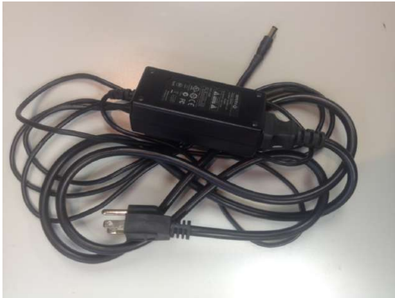
Figure 3: Power Supply (12 VDC)
