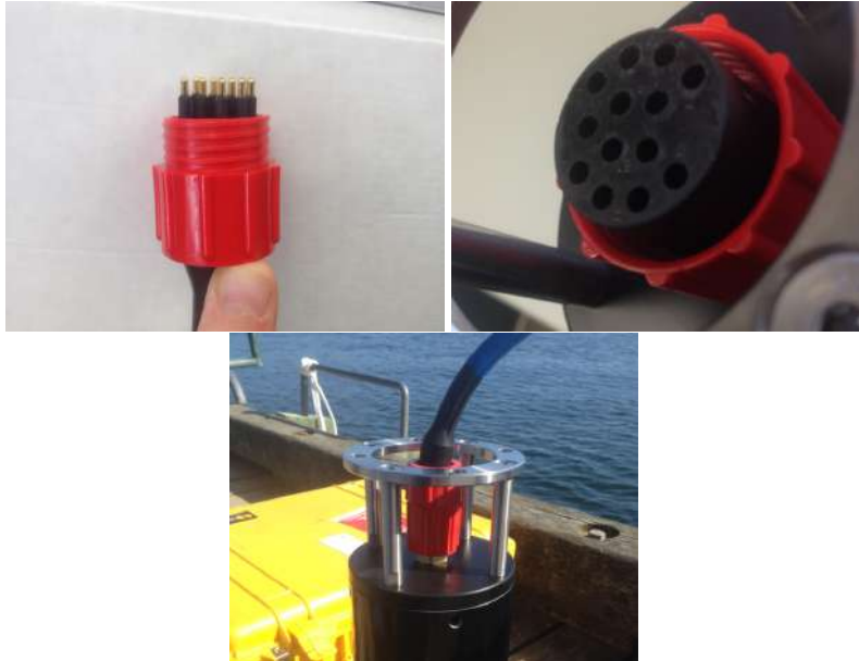
Figure 9: Locking sleeve on both the cable (left panel), the microscope (center panel) and connected (right panel)
