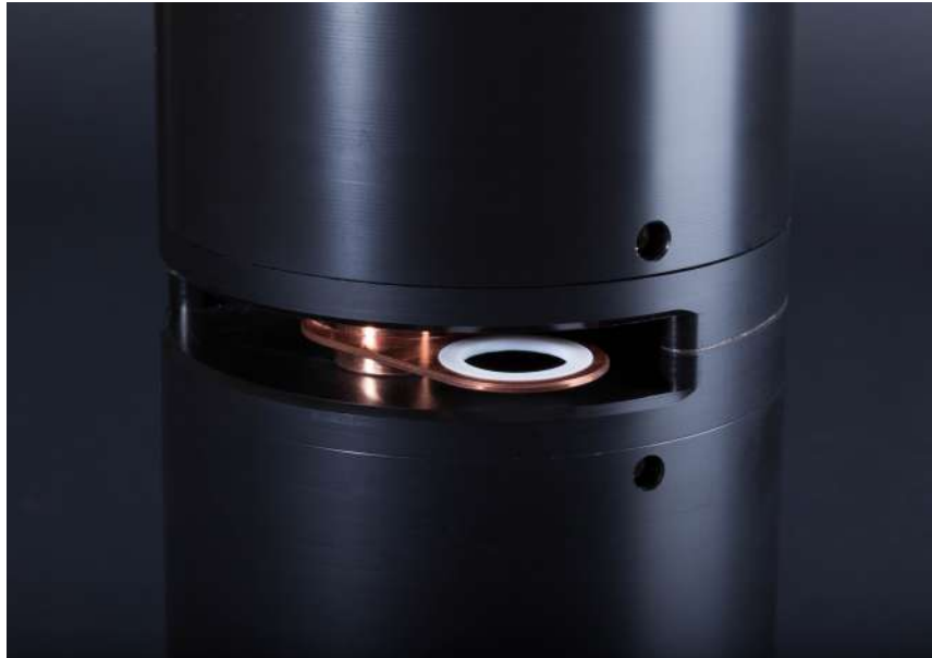
Figure 6: The sample delivery system, containing the white washer and copper, to reduce biofouling.
