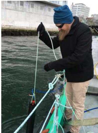
Figure 26: Deployment of the FluoroSea from a stationary ship on a wharf
