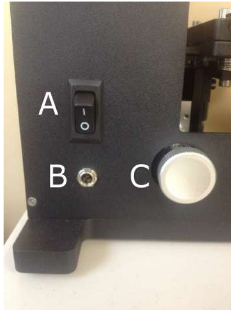
Figure 11: The Z- control knob for the sample stage (object “C”).
