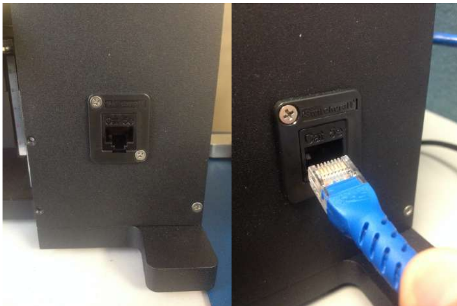
Figure 7: The Ethernet cable port on the microscope (left panel). Plugging the Ethernet cable into the microscope port (right panel).
