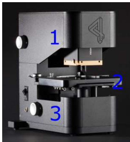
Figure 9: Main view of the Desktop microscope, showing 1) the camera housing, 2) the sample stage and 3) the point source
