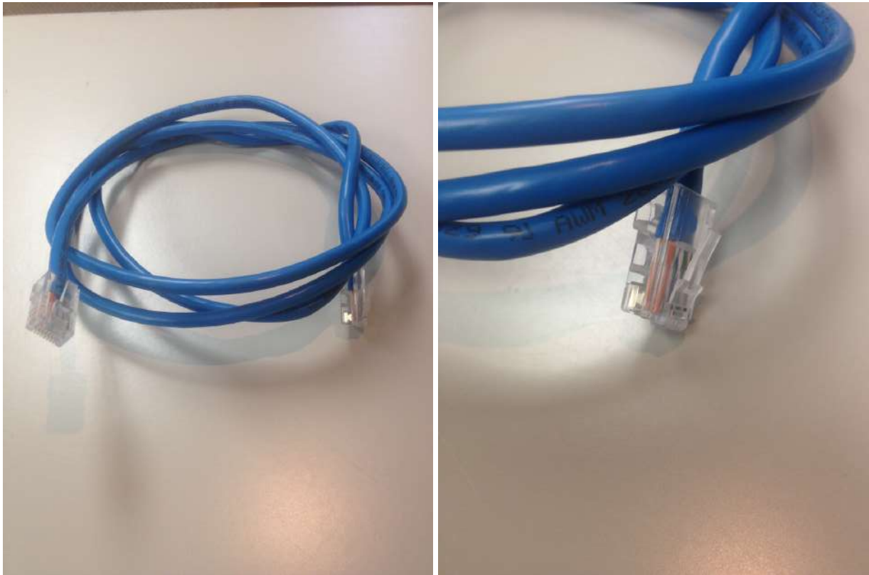
Figure 3: Ethernet cable from a distance (left panel) and close-up (right panel) of the connector
