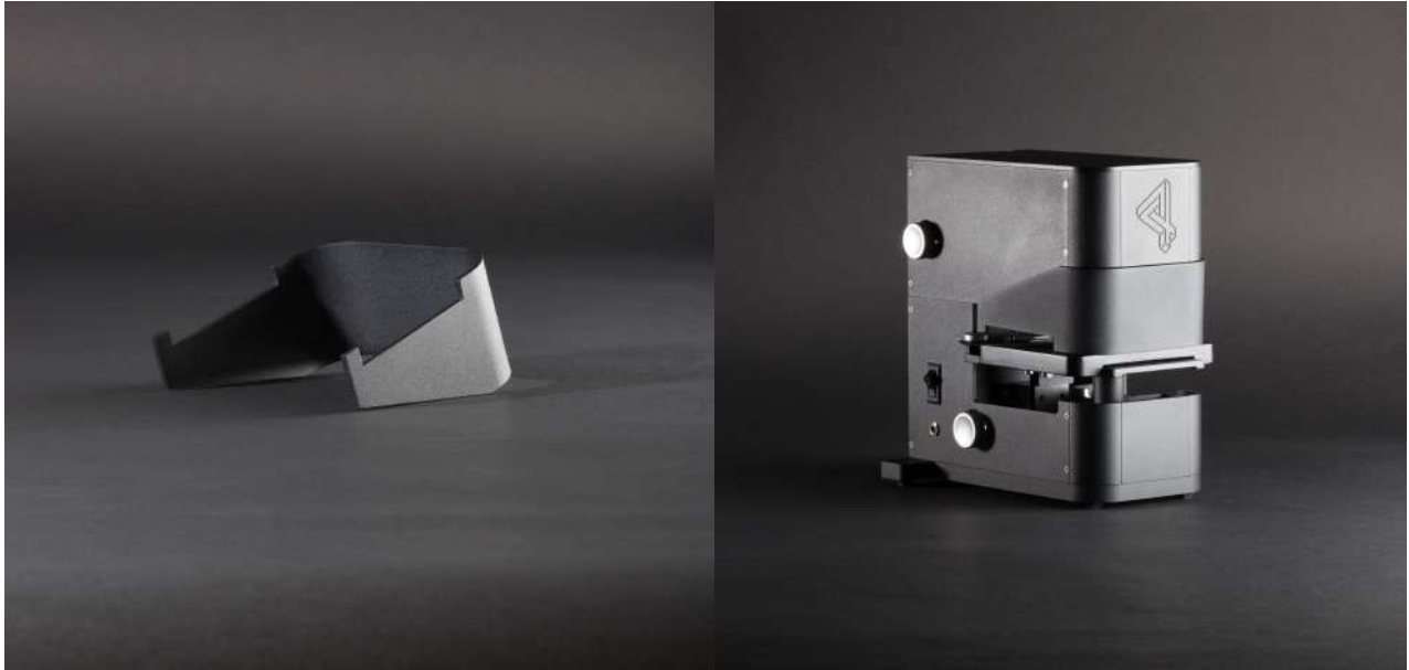
Figure 5: Desktop shield (left panel) and Desktop microscope with shield in place (right panel)
