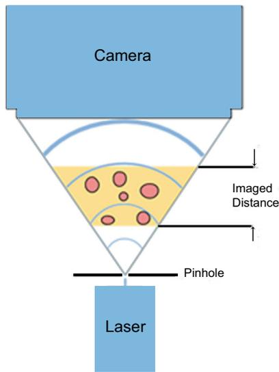
**Figure 1** Schematic of the DIHM set-up used in this study. In our case, the laser has a wavelength of 400 nm and a single mode optical fibre of 1.6  $\mu\text{m}$  diameter replaces the pinhole.
