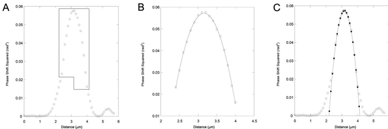
**Figure 3** (A) Square of a phase profile obtained by taking a radial cross section from a phase reconstruction of one hologram. (B) Data points within the region indicated in (A) are fit using Eq. (1). (C) The fit plotted together with the entire squared phase profile. The flaring at the edges of the fibre is due to the point spread function of our instrument.
