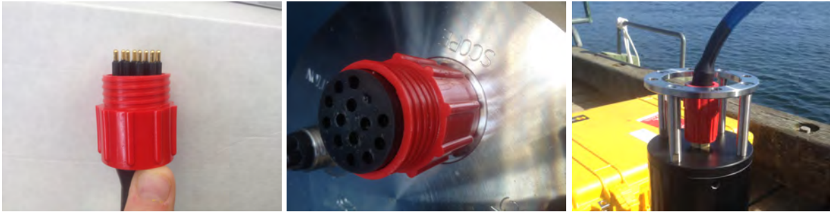
Figure 11: Locking sleeve on both the cable (left panel), the microscope (center panel) and connected (right panel)
