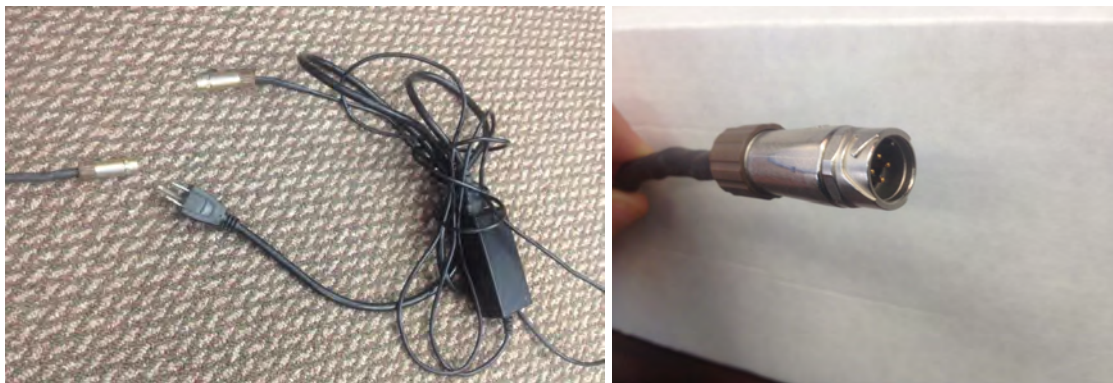
Figure 14: Connecting the power. In the left panel connecting the microscope power to the included 12VDC power cord. The right panel shows a close-up of the power connector from the microscope.
