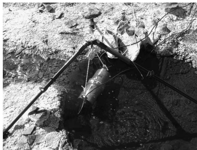
**Fig. 3.** Photo of the DIHM instrument suspended from a tripod over spring GH4.
