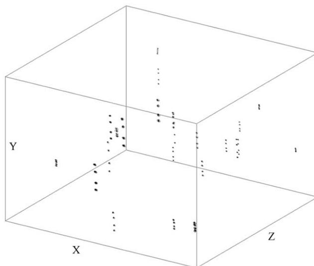
**Fig. 4.** Reconstructions of a sequence of four holograms taken in the water of spring GH4. The 3-D representation of the particle trajectories was obtained from 100 reconstruction planes and the image demonstrates the large depth of field that can be achieved with DIHM. The majority of particles were moving upward at 16 μm/s and can be identified as detritus. Distances: X = 480 μm, Y = 480 μm, Z = 2250 μm. Exposure time: 65 ms; 4 f/s.
