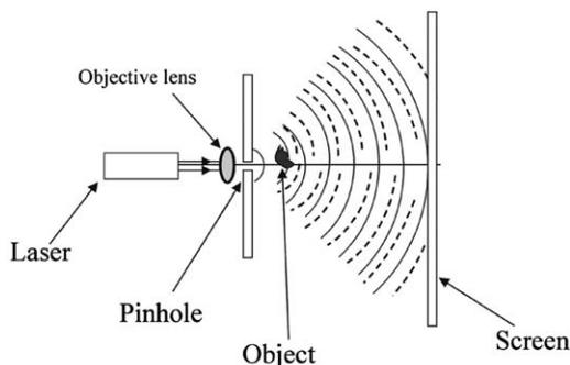
Fig. 1. Principle of digital in-line holographic microscopy.
