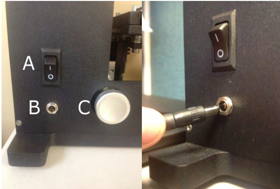
Figure 6: Power port shown as object “B” in the left panel. Plugging the power cable into the microscope port (right panel).
